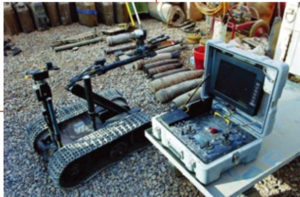
The TALON combat-ready robot, developed from platforms funded by several DARPA SBIR Awards
